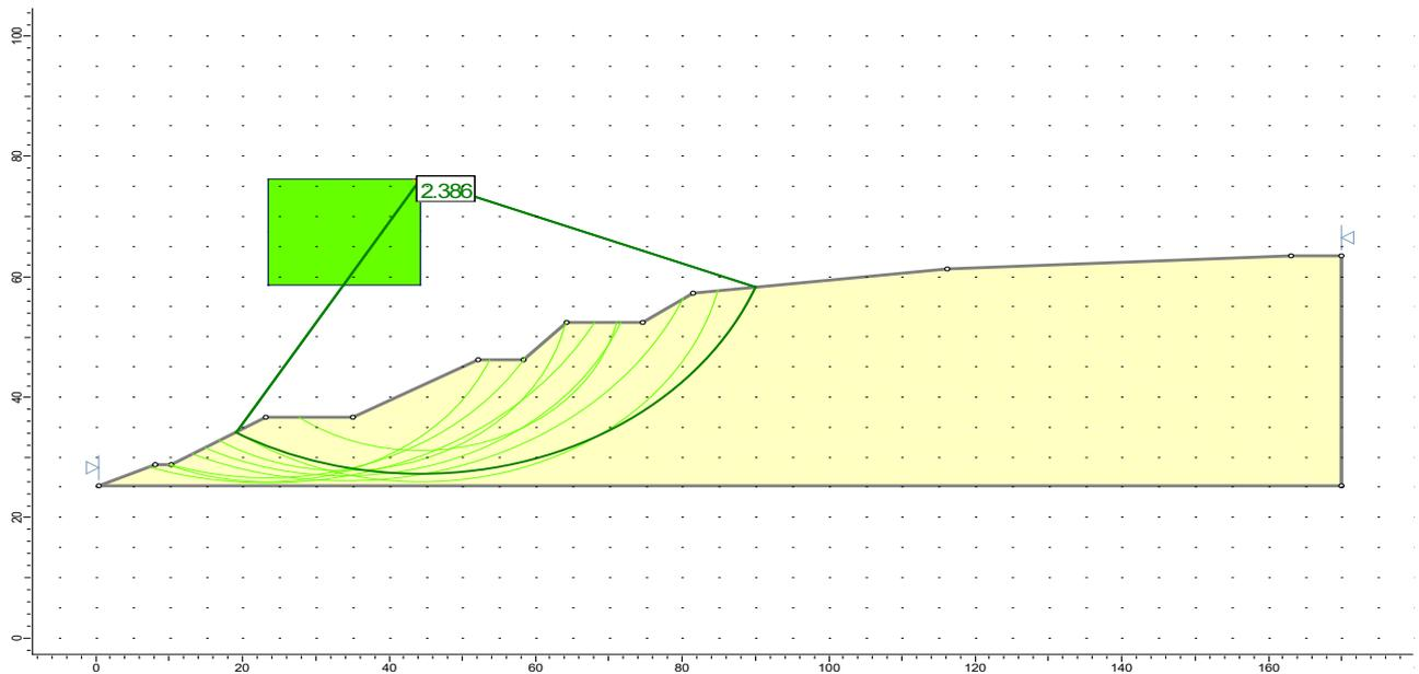
Figure 2 – Minimum shear surfaces and global minimum stability factor based on the results of the calculation for section 3-3 (left slope)
