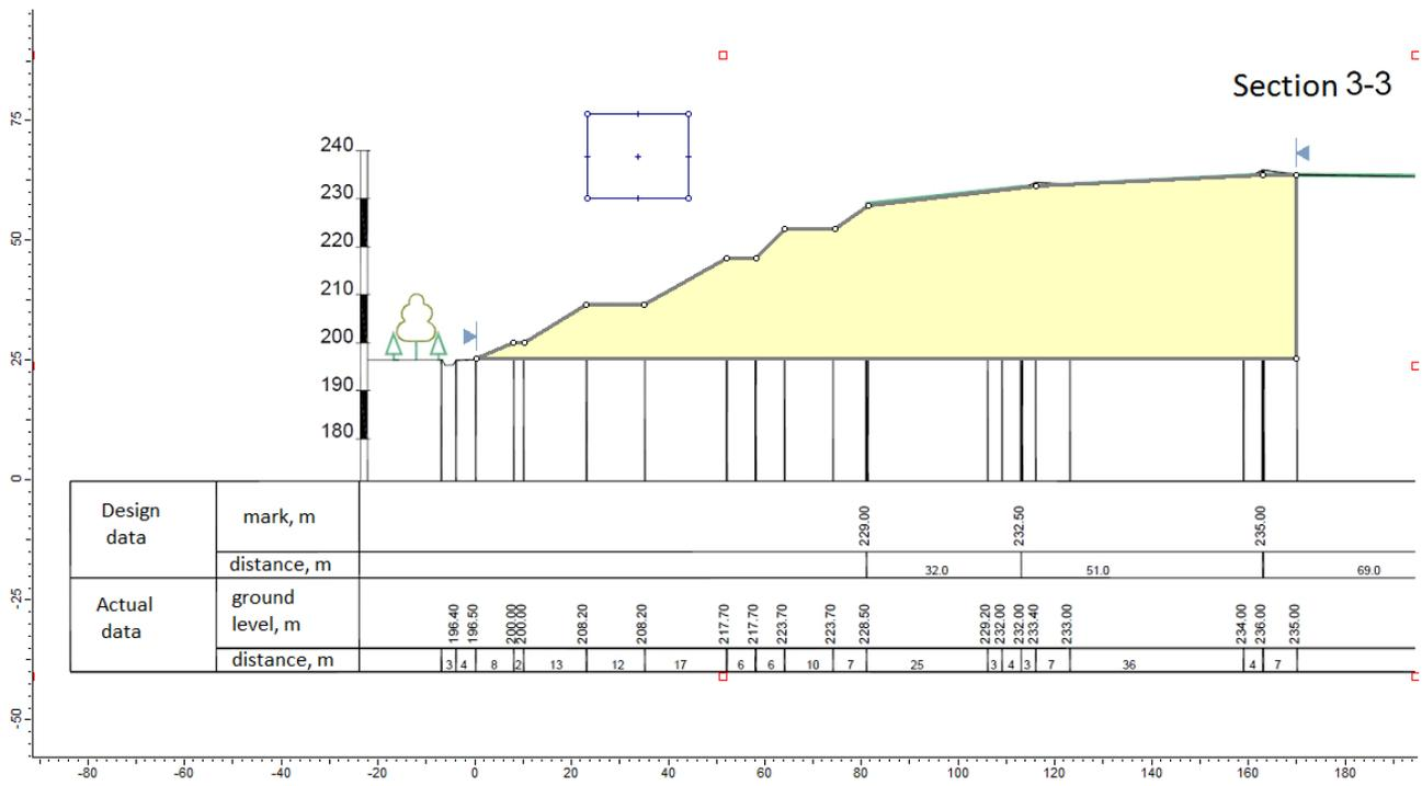
Figure 1 – Design scheme for the calculation of section 3-3 (left slope)
