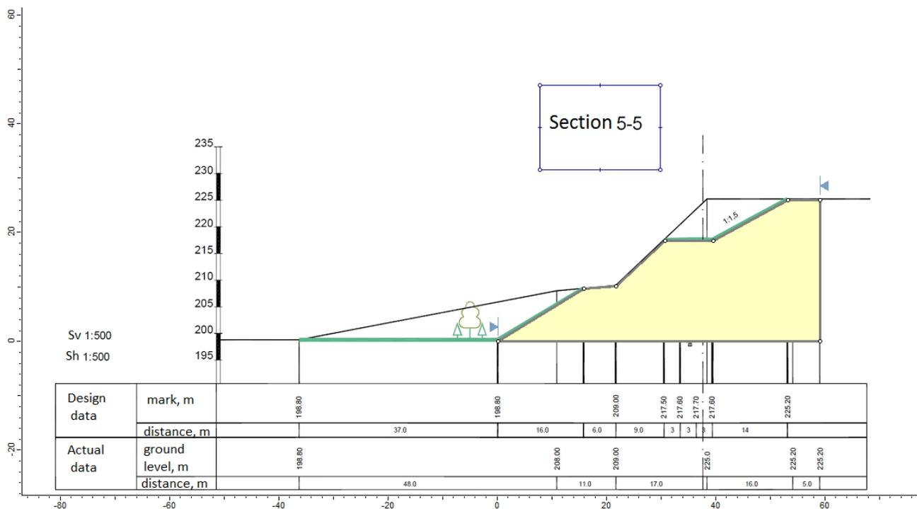
Figure 4 – Design scheme for the calculation of section 5-5
