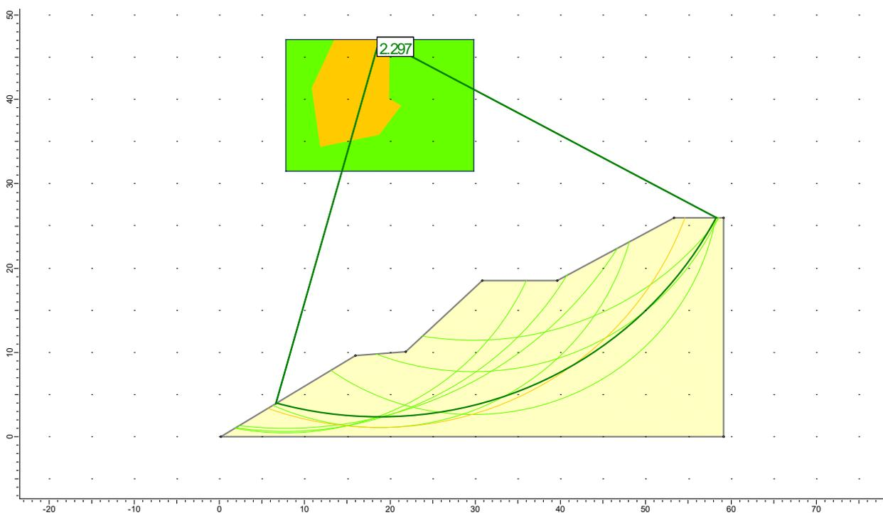
Figure5 – Minimum shear surfaces and global minimum of the stability factor based on the results of the calculation in section 5-5
